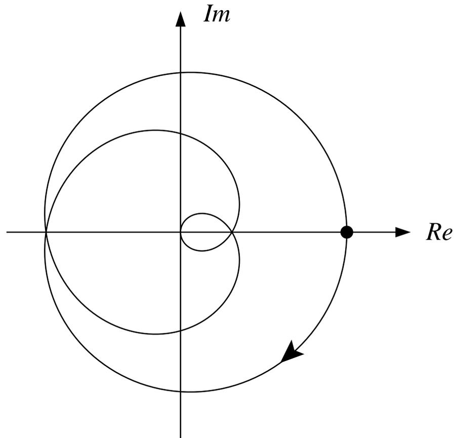
**Figure 6.** The path described in the complex plane by the frequency-response function  $\psi(\omega)$  of the differencing filter  $\psi(L) = L^2 - L^3$  as  $\omega$  increases from  $-\pi$  to  $\pi$ . The trajectory originates in the point on the real axis marked by a dot. It traverses the origin when  $\omega = 0$  and it returns to the dot when  $\omega = \pi$ .
