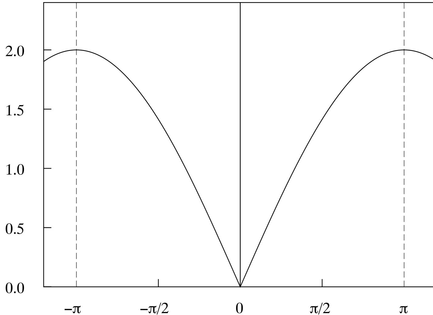
**Figure 7.** The gain  $|\psi(\omega)|$  of the differencing filter  $\psi(L) = L^2 - L^3$ .
