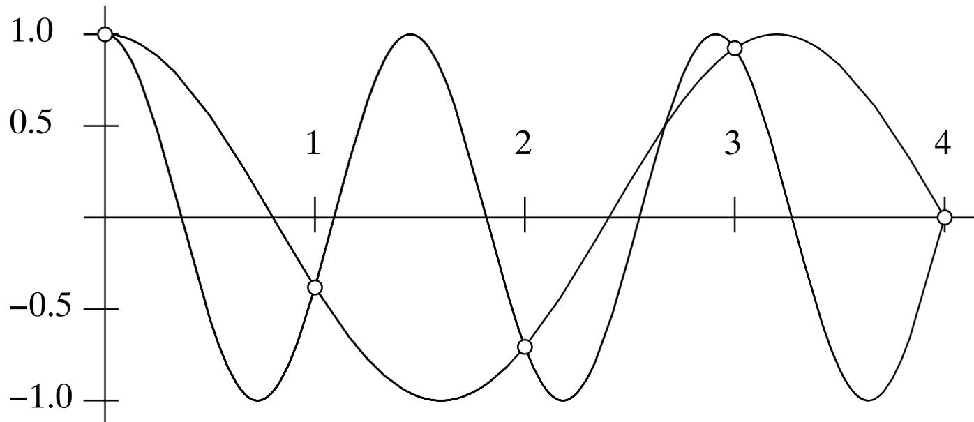
Figure 11. The values of the function  $\cos\left\{\left(\frac{11}{8}\right)\pi t\right\}$  coincide with those of its alias  $\cos\left\{\left(\frac{5}{8}\right)\pi t\right\}$  at the integer points  $\{t = 0, \pm 1, \pm 2, \dots\}$ .
