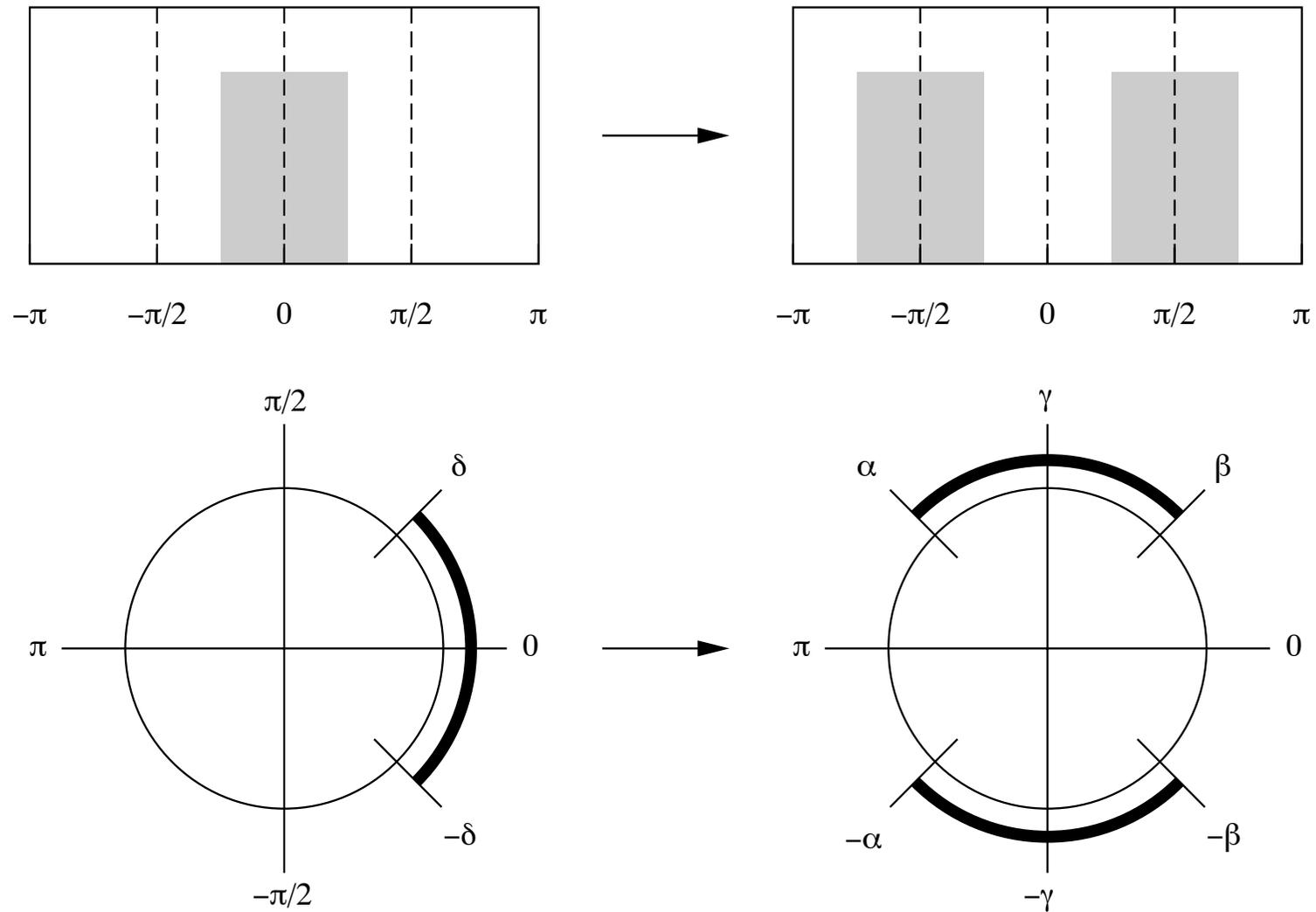
**Figure 9.** The conversion of a lowpass filter to a bandpass filter by a cosine modulation, which creates two copies of the lowpass filter.
