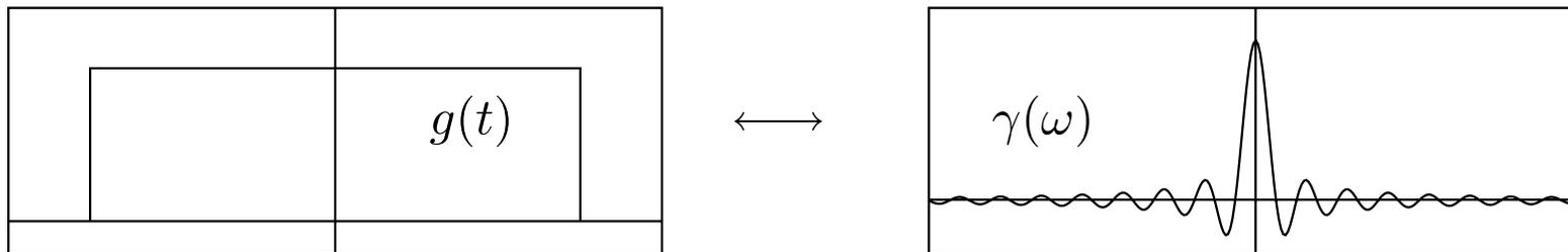
The Fourier Transform of a time-domain rectangle is a sinc function in the frequency domain.
