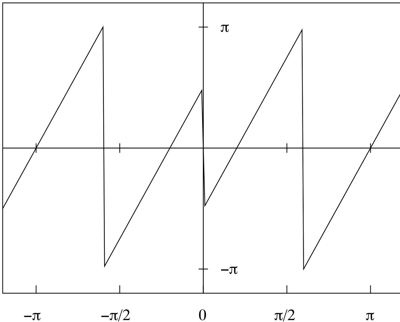
**Figure 8.** The phase  $-\text{Arg}\{\psi(\omega)\}$  of the differencing filter  $\psi(L) = L^2 - L^3$ .
