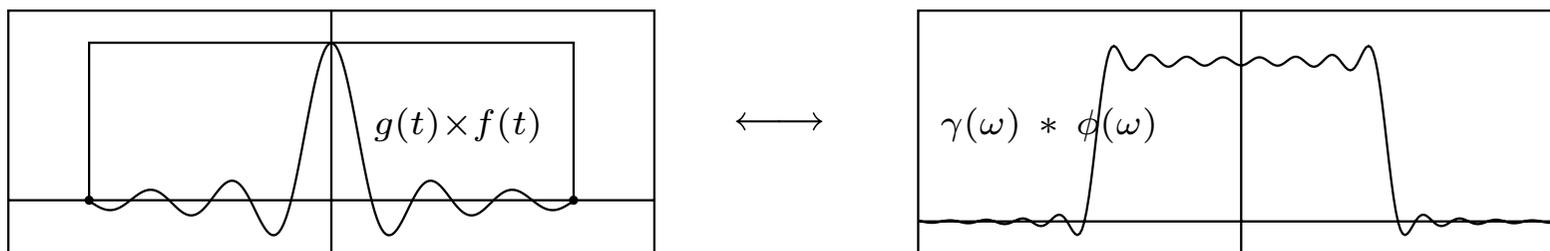
Truncating the time domain sinc function causes leakage in the frequency domain. The time-domain truncation corresponds to a convolution in the frequency domain.
