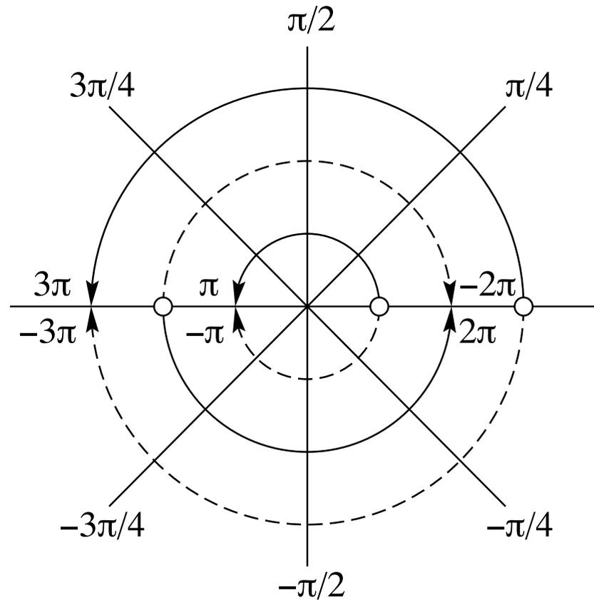
**Figure 12.** A diagram to illustrate the aliasing of frequencies when the Nyquist frequency is at  $\pi$  radians per sample interval. The arcs with the broken lines correspond to negative frequencies.
