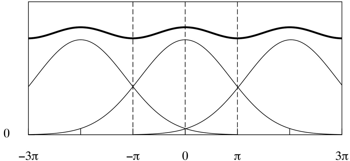
**Figure 13.** The figure illustrates the aliasing effect of regular sampling. The bell-shaped function supported on the interval  $[-3\pi, 3\pi]$  is the spectrum of a continuous-time process. The spectrum of the sampled process, represented by the heavy line, is a periodic function of period  $2\pi$ .
