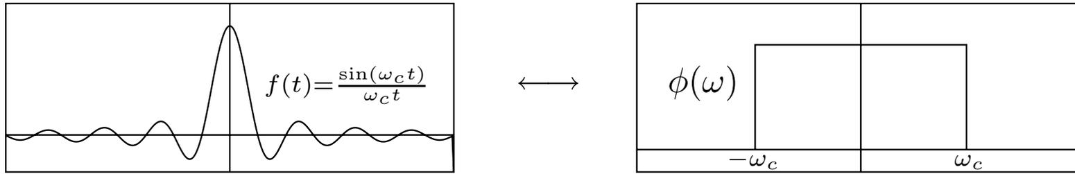
The Fourier Transform of a time-domain sinc function is a rectangle in the frequency domain.
