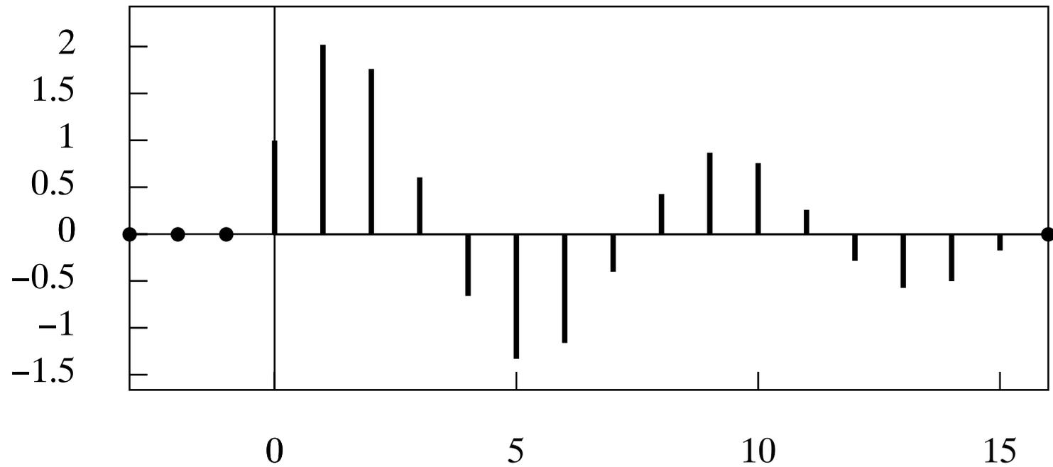
**Figure 5.** The impulse response of the transfer function  $\theta(z)/\phi(z)$  with  $\phi(z) = 1.0 - 1.2728z + 0.81z^2$  and  $\theta(z) = 1.0 + 0.75z$ .
