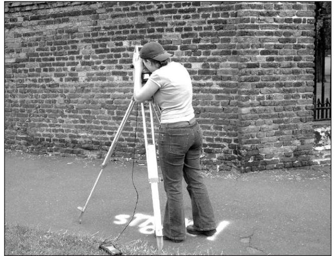
*Above:* Surveying the diaper patterns on the wall using a reflectorless total station electronic distance measurer.
