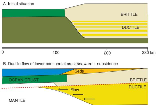
Fig. 5. After the initial rifting the lower crust deforms by plastic flow. Could the lower continental crust flow UNDER oceanic crust in the manner shown?
