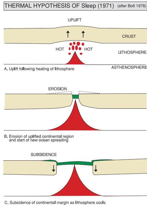
Fig. 3. Thermal hypothesis of Sleep. This was the first to recognise that heating up the mantle (by a plume or whatever) could produce substantial crustal uplift (and erosion), followed by thermal subsidence. Compare the models by McKenzie and Wernicke later . .
