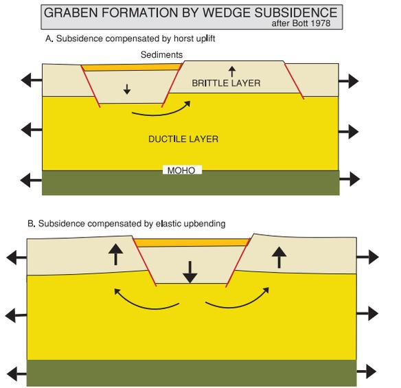
Fig. 7. Can normal faulting lead to displacement of ductile mantle by flow?
