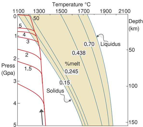
Fig. 14. With pure shear the temperature of the uprising asthenosphere can exceed the solidus of the mantle and allow melting.
