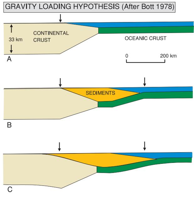
Fig. 2. Gravity loading hypothesis. This depends on replacing low density water by higher density sediment . . .
