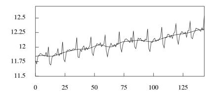
Figure 11: The logarithms of U.S. total retail sales from January 1953 to December 1964 with an interpolated trend-cycle function.
