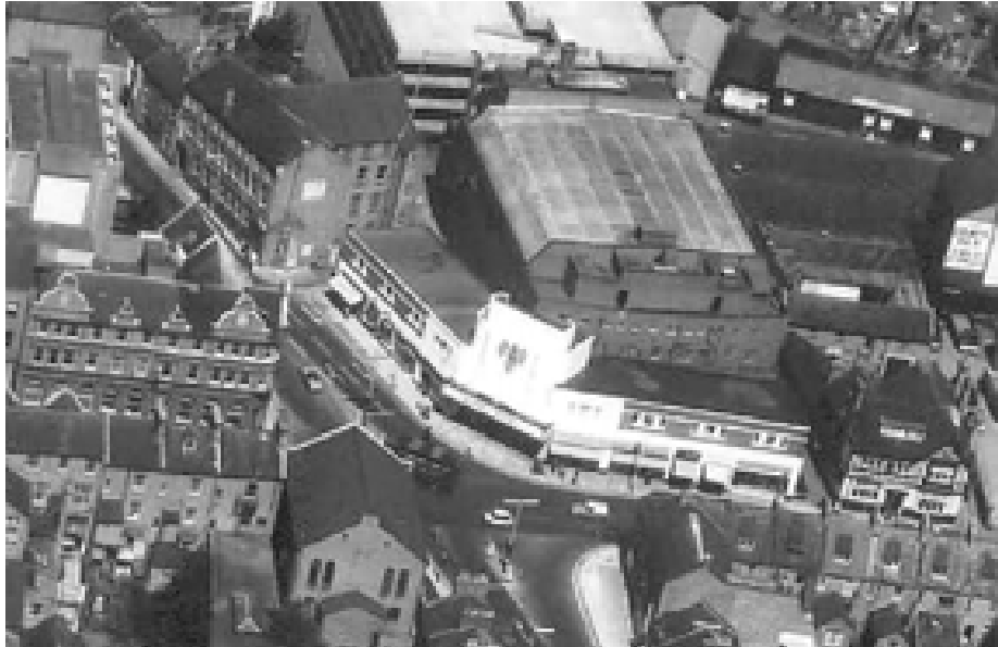
Fig. 20 Aerial view of cinema. Projection room can be seen on the rear part of the auditorium roof. (Jesus army Web Site)
