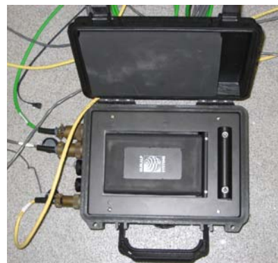
Figure 1: A standard Guralp DCM module
