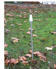
Figure 3: The modem antenna for one of the new systems
